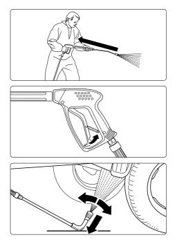
Bear in mind that during cleaning tasks with a high-pressure water jet a significant recoil at the lance arises. Additionally angled lances produce a clearly perceivable amount of torque.
