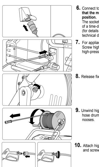
6. Connect to power circuit. Make sure that the main switch is on the "OFF" position.
