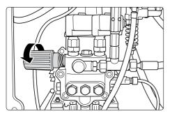
The operating pressure, the water flow and correspondingly the water temperature ist controlled by the pressure control valve.
