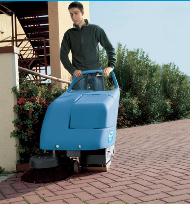
Dirt is conveyed straight into the hopper which is strong and lightweight for easy handling
