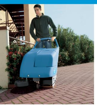
Dirt is conveyed straight into the hopper which is strong and lightweight for easy handling
