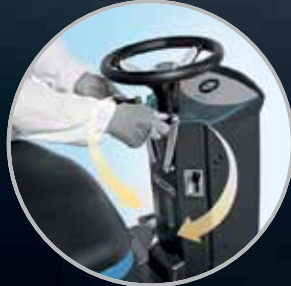
Turn on water and lower the brush head and the squeegee
