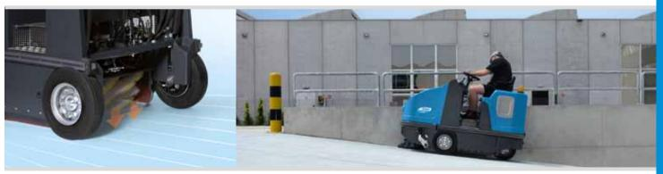
The central brush is the floating type and self-adjusts to keep in contact with the ground all the time
