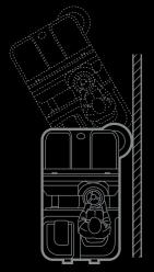
The body with rounded edges and protected by a rubber profile improves sweeper manoeuvrability
